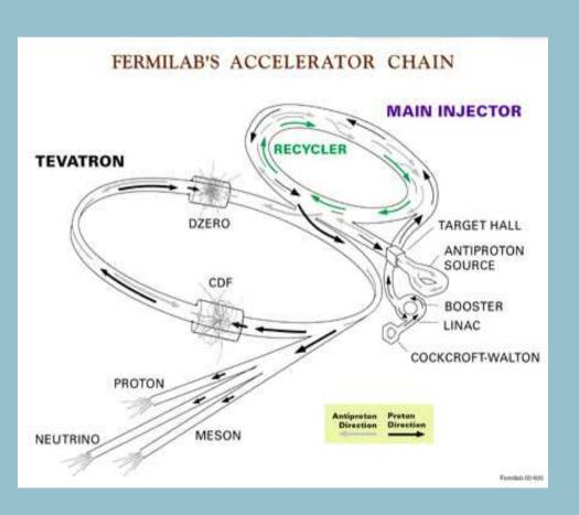
The Tevatron, with a center of mass energy of 1.96 TeV, was the most power accelerator in the world. It collided protons with anti-protons every 396 ns.
