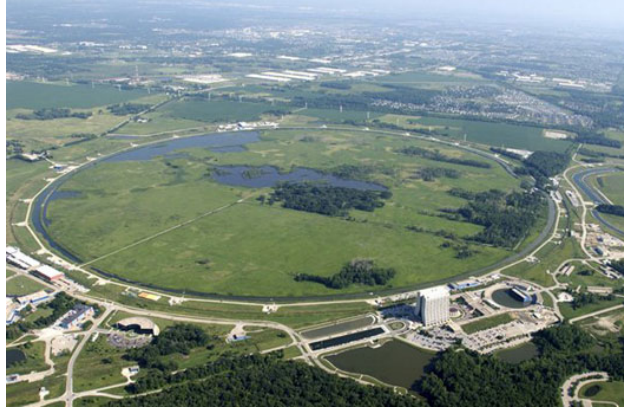
Fig. II.1. Aerial view of the Fermilab site with a clear view of the ring next to Wilson Hall (which is the tall building in the foreground). The Tevatron sits underground just outside of the service road shown here. There are two places the beams are brought to collide called the Collision halls. There aren't distinguishable in this picture but there is one on the close side housing the CDF detector and one on the far side housing the D0 detector.[14]
