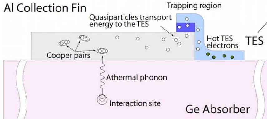
The TES response changes the current in the channel (each channel is 455 QETs connected in parallel). The current is coupled to a SQUID to get out of the cryostat, and amplified in the front-end electronics. We use the change in current relative to a stable baseline to measure the phonon energy.
